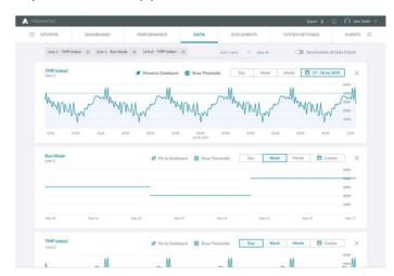
Presenting entire weeks or months of multiple graphs gives a good overall picture. In addition, process details become directly visible with the simple zoom function via a click of the mouse.
