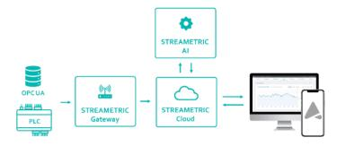
Our experts will support you with the interface definition and a trouble-free installation, remotely or on-site. Once the system is connected, users can access the portal on all devices with a web browser. STREAMETRIC is a software-as-a-service. This means regular service and updates are available after installation.
